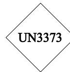
Biological Substances, Category B
