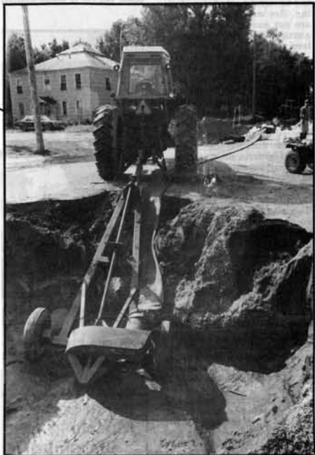
A power take off pump at Route 78 was used to lift water over the highway from a ditch in Bath. One-third of the village was under water Tuesday.
